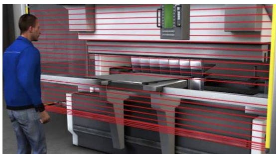
Fig 30: Power press equipped with a safety light curtain, fixed enclosure guard, two-hands activation control and an emergency stop and shrouded foot paddle
