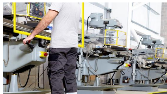
Fig 38: Safety trip control
