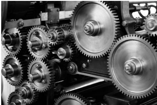
Fig 17: In-running nip points
