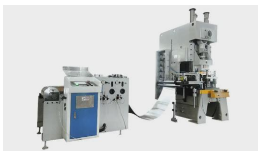
Fig 26: Power press with automatic feed
