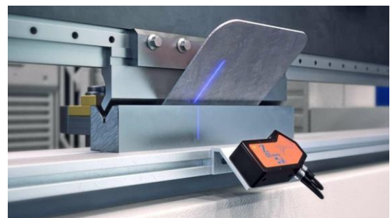
Fig 31: Press brake installed with laser sensing system that has transmitter and receiver mounted below the RAM to cut off power supply to prevent hand and finger injuries
