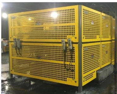
Fig 19B: Typical guard for tail section of a conveyor
