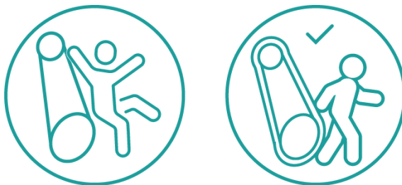
Fig 13: Un-guarded machine hazard and control measure
