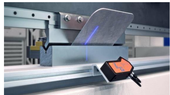
Fig 31: Press brake installed with a laser sensing system that has transmitter and receiver mounted below the RAM to cut off the power supply to prevent hand and finger injuries
