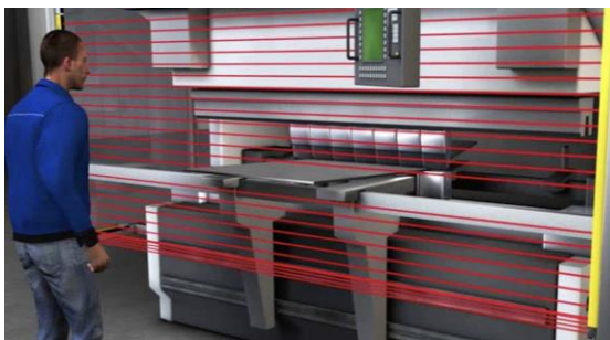
Fig 30: Power press equipped with a safety light curtain, fixed enclosure guard, two-hand activation control, and an emergency stop and shrouded foot paddle
