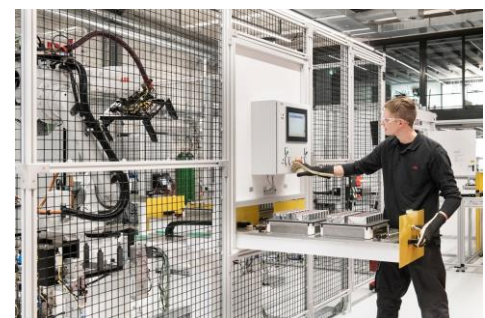
Fig 39: Shows a typical robot work cell safeguarding system
