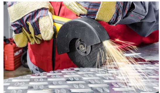
Fig 29: Grinding machine protection with plastic or metal cover to avoid flying chips
