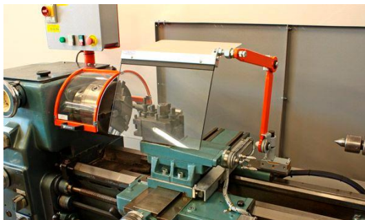
Fig 28: Lathe machine protection with plastic cover to avoid flying chips
