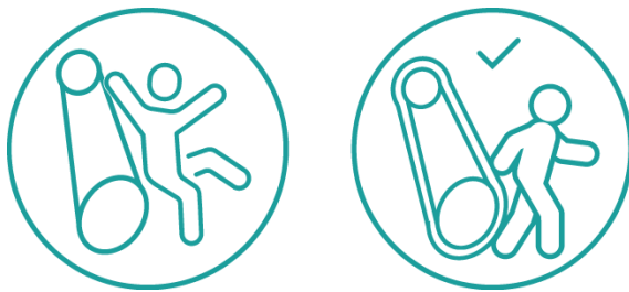
Fig 13: Un-guarded machine hazard and control measure
